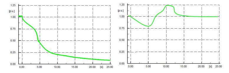
Simulations showed Santerno power management solution to be extremely effective at stabilizing the local grid even during the most demanding transients thanks to the combined effect of fast active power and reactive power modulation.
