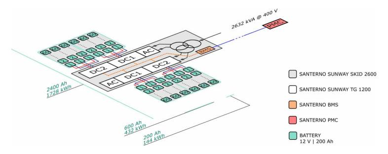
High level power management control is implemented at the PMC level. Santerno PMC features include voltage regulation, P/Q setpoint, power shift, frequency feedback control. Medium level battery management is implemented at Skid level, thanks to Santerno BMS. BMS features include battery supervision, charge/discharge, periodic equalization. Low level power conversion control is embedded into the inverters and includes grid interface functions, power regulation, voltage feedback control.
