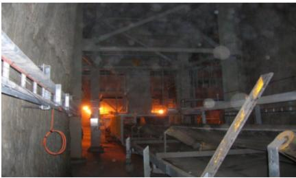
...where, through a 300m conveyor (one 500 kW motor) is conveyed at the surface level and sent to the main conveyor belt.
